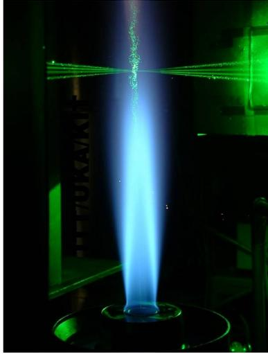
FIGURE 1.2. Turbulent Premixed Flame
