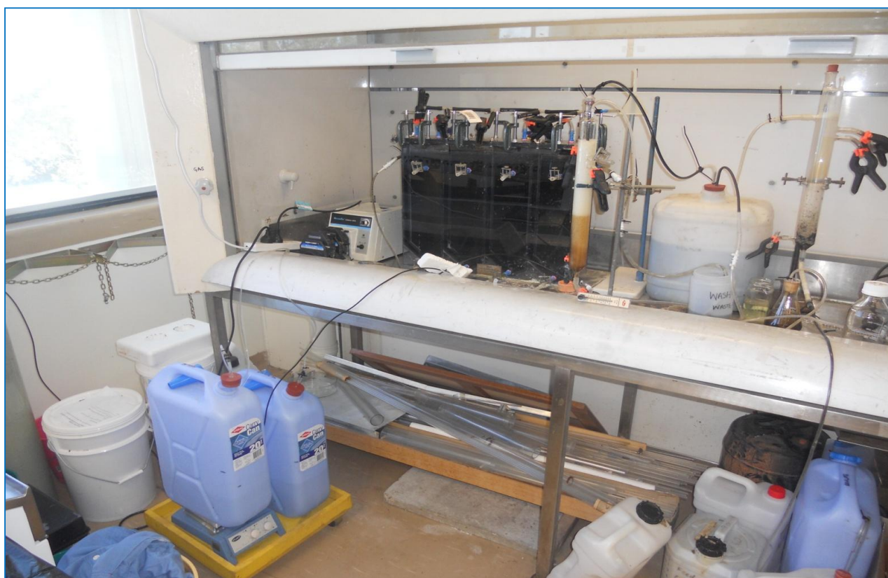
Figure 20.5 Photograph of anaerobic baffled reactor (ABR).
