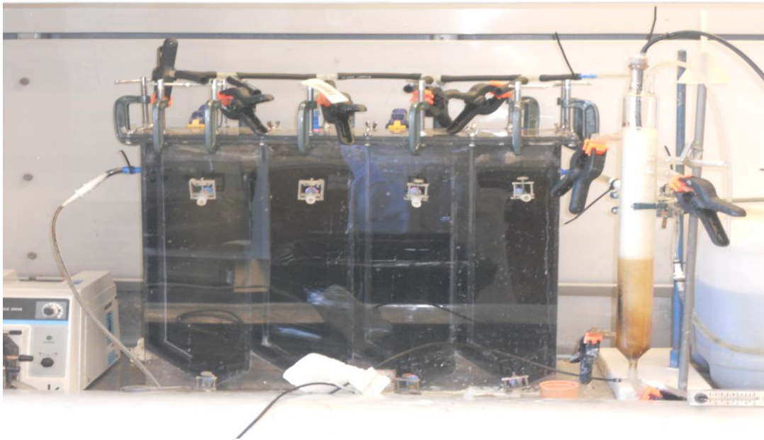
Figure 4.4. Photography of anaerobic baffled reactor during the experiment; on the right side is showed also the separated column precipitation reactor.
