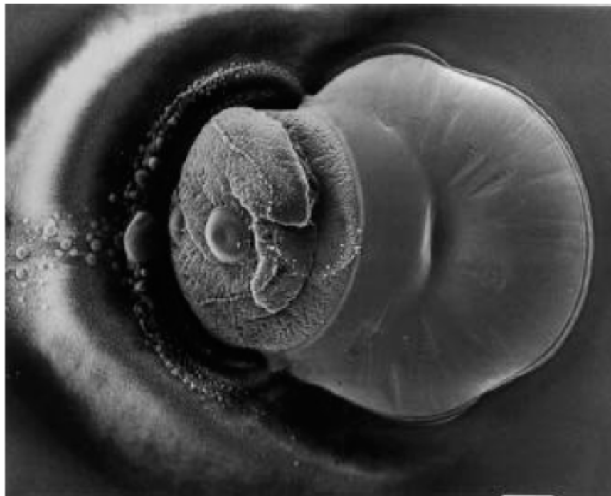
Fig. 93 – Example of Al particle partially incorporated in the oxide residual
