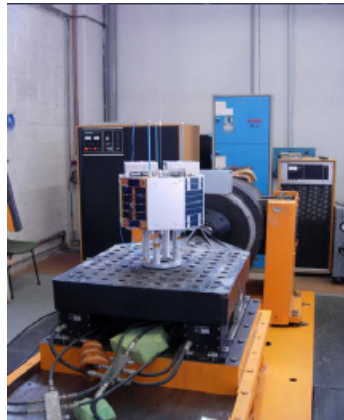
Fig. III-20. UNISAT-4 vibration test.
