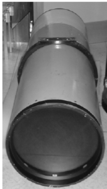
Fig. IV-8. 30 cm Baker-Schmidt optical tube (Ref. 47).
