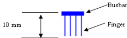
Fig. III-2. Technique of solar cell assembly on the sun sensor.
