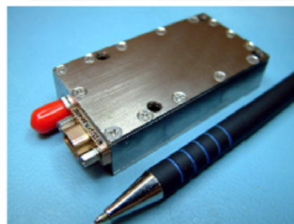
Fig. III-33. UHF, VHF transceiver and S-Band transmitter.
