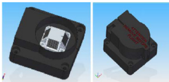
Fig. III-5. CAD drawing of solar sensor assembly (left side) and the solar sensor with the cover (right side).
