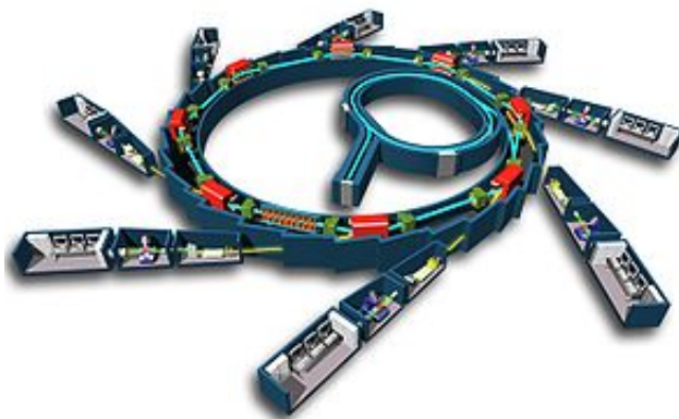
Fig. 2.5.1 Scheme of synchrotron radiation facility
