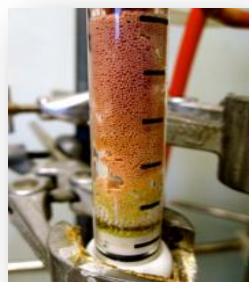
Figure 29. Succinimide trapped on Ambersep 900 (strong basic ion-exchange resin).
