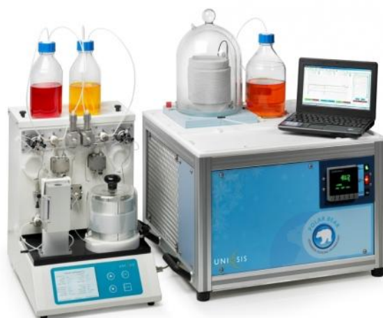
Figure 7. Polar Bear reactor developed by Cambridge Reactor Design (CRD) and connected to a Uniqsis FlowSyn platform, used to run reaction under cryogenic conditions
