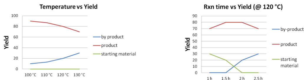
Figure 15. Relationship between yield and temperature in batch reactions
