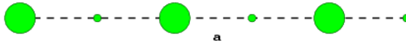
Figure 2.1: A 1-dimensional charge density wave; it represents a kind of variant. The radius of the circles is proportional to the charged density.
