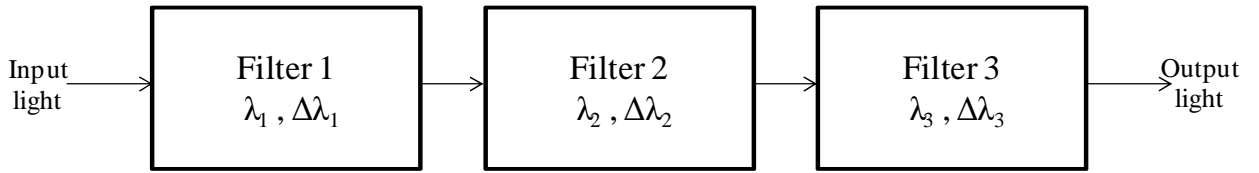
Figure 3.13: Series of optical filters.
