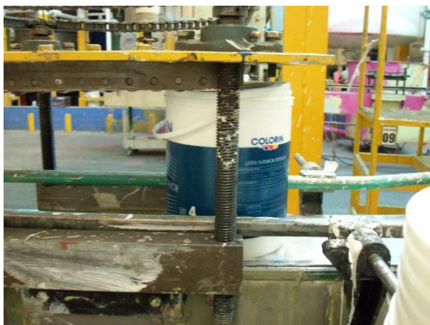
Figure 4.4.20: Plastic packaging spotted due to filling machine bad cleanness condition (Left side)
