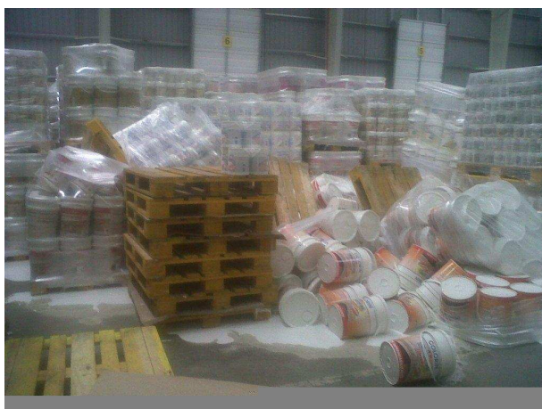
Figure 4.2.10 and 4.2.11: Fallen pallets, leakage and waste material losses even with standardized pallet
