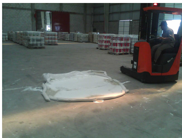
Figure 4.2.6 and 4.2.7: Distribution center deficient truck loading due to use of unstandardized pallet
