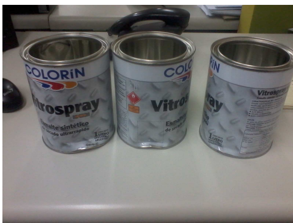
Figure 4.4.22: One liter can with bottom dented due to incorrectly stacked and stowed (Left side)
