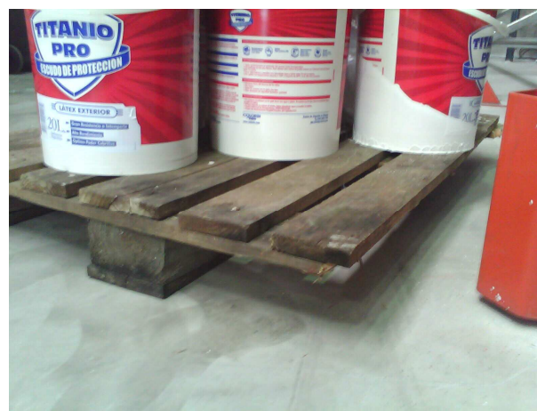
Figure 4.2.6 and 4.2.7: Distribution center deficient truck loading due to use of unstandardized pallet
