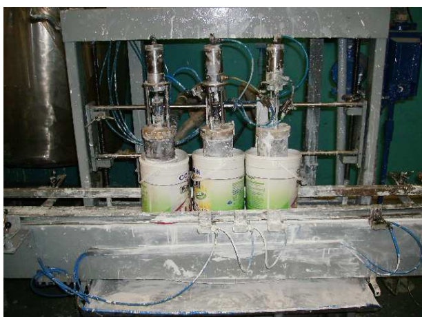
Figure 4.4.18: New plastic packs used for filling machine setting (Left side)
