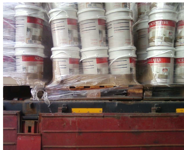
Figure 4.2.6 and 4.2.7: Distribution center deficient truck loading due to use of unstandardized pallet
