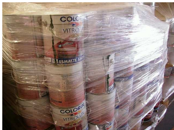
Figure 4.4.20: Plastic packaging spotted due to filling machine bad cleanness condition (Left side)
