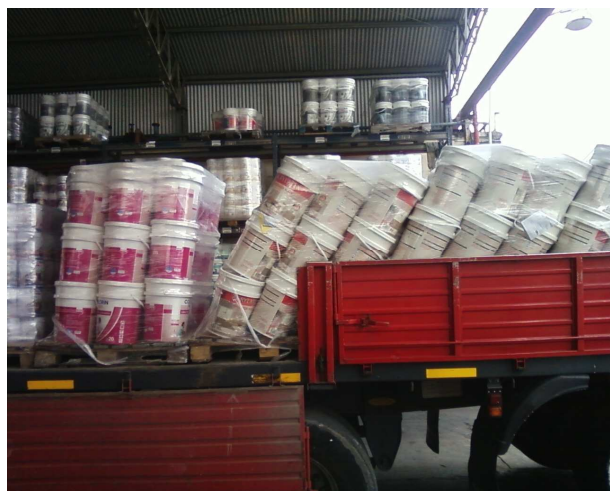
Figure 4.2.6 and 4.2.7: Distribution center deficient truck loading due to use of unstandardized pallet
