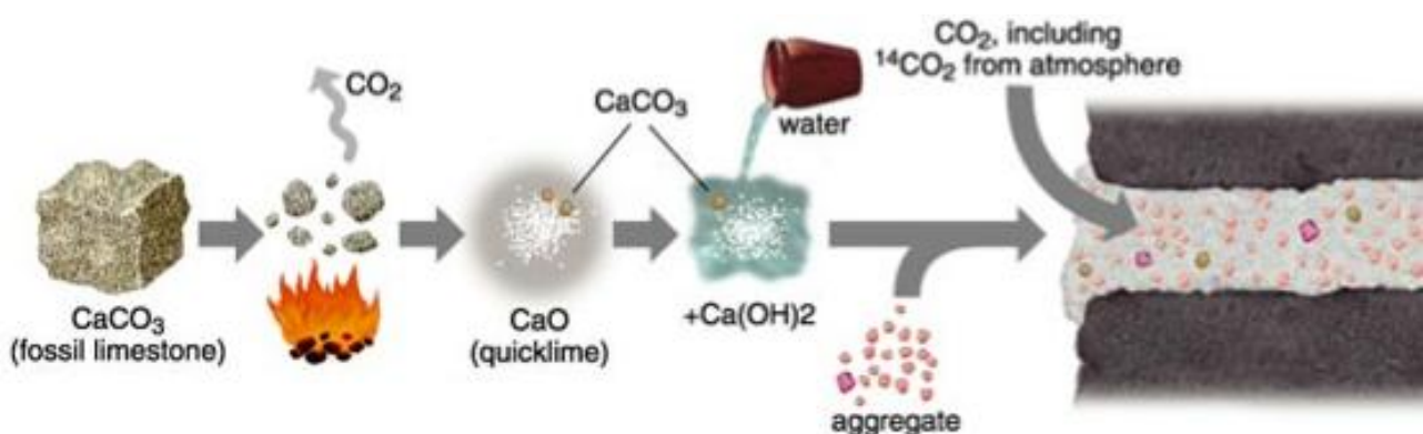
Figure 1. The \text{CaCO}_3 cycle from limestone to binder calcite presented schematically (Hale et al.2003).
