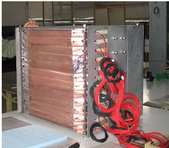
Figure 3.39: A picture of the GGM system ready to be shipped to CERN. The stack is enclosed into an aluminum box for further shielding.
