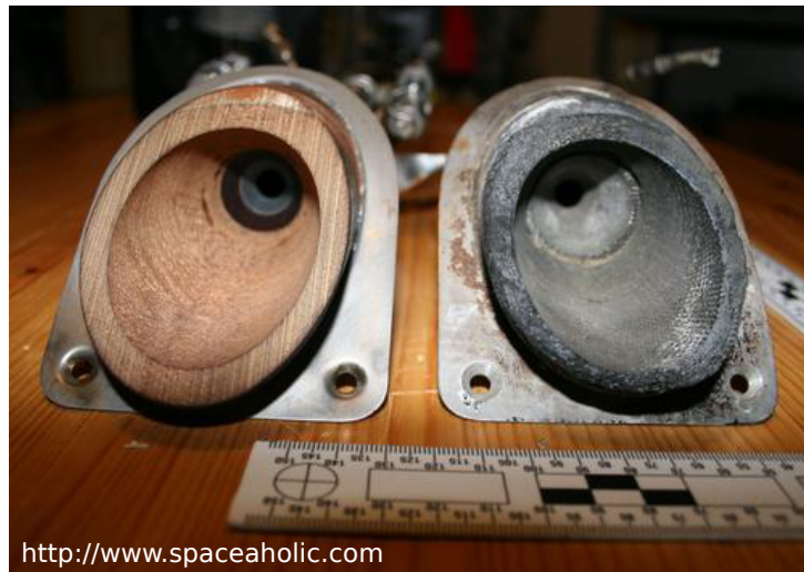
Figure 1.1 – Comparison of silica-phenolic nozzles before and after firing.
