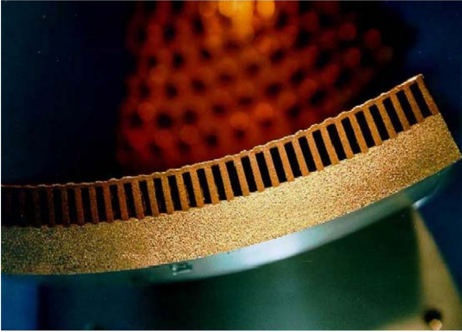
Figure 1.8: Cut through a combustion chamber wall with CuAgZr liner and galvanic deposited Ni outer shell. Taken from [50].
