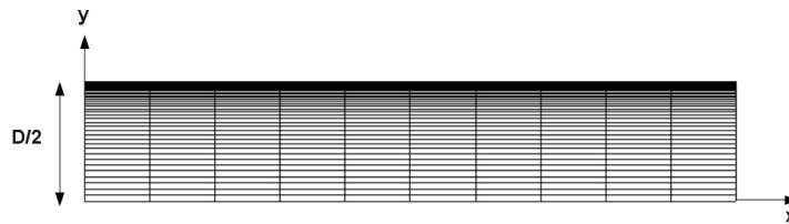
Figure E.2: Projection of the two dimensional axisymmetric grid a plane containing the symmetry axis
