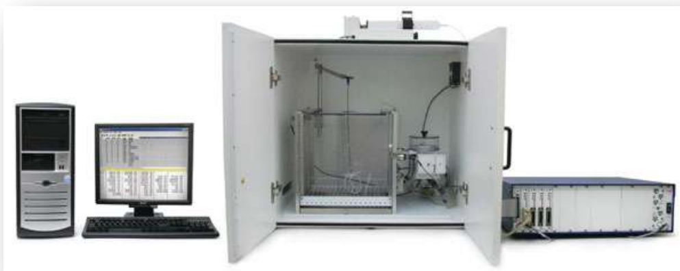
Picture 16 Each operant-chamber is placed within a cubicle, connected either to a syringe pump, throughout an electronic interface, and to a computer software. [ www.med-associates.com/drug_del/rmouseselfadmin.htm ]
