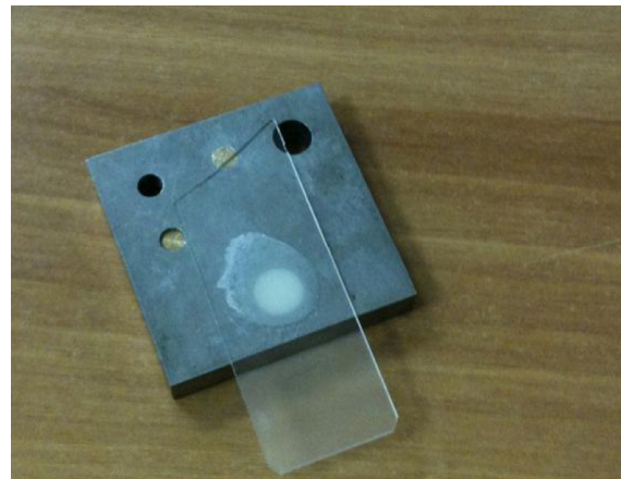
Figure 3. Glass plate application over the cylindrical metal matrix with exceeding material.
