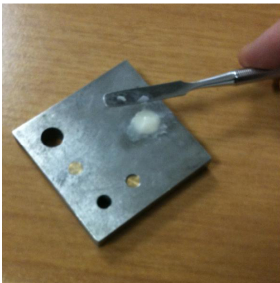
Figure 2. The material was applied in the cylinder in the remaining depth.
