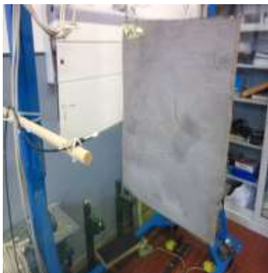
Fig. 11 Acoustic test set-up, Plate with Foam 65-30
