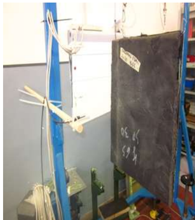
Fig. 10 Acoustic test set-up, Plate with Original Foam
