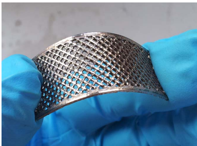
Figure 8. NiP plated PETG flexible demonstrator.
