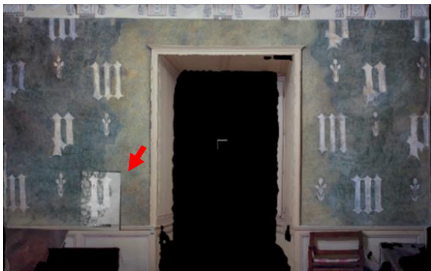
Figure 15: Snapshot from the SIVT application tested on Germolles case study data. The rectified and registered IR image of the “P” (red arrow) is displayed on top of the orthophotograph of room dn south wall ©Wefers and Reich.
