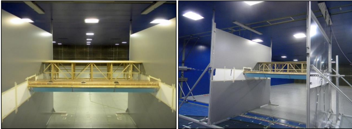
Figure 3. Pictures of the sectional models in wind tunnel during static and dynamic tests
