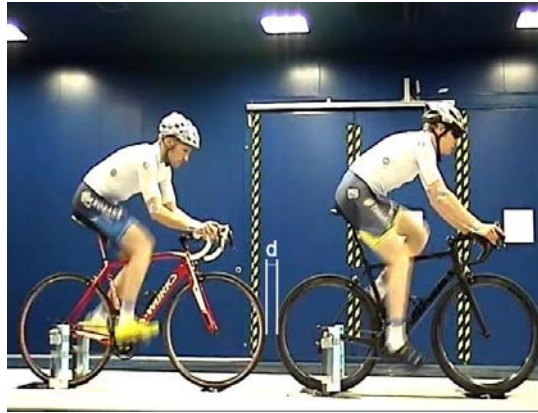
Figure 1. Cyclists layout in the wind tunnel. The distance d between the bikes is highlighted
