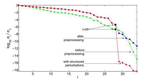
Fig. 4. The normalised singular values  $\sigma_i/\sigma_1$  of the Sylvester matrix of (i) f(y) and  $g(y) \blacksquare$  (before preprocessing), (ii)  $\bar{f}(w)$  and  $\alpha_0 \bar{g}(w) \bullet$  (after preprocessing), and (iii)  $\tilde{f}(w)$  and  $\beta^* \tilde{g}(w) \bullet$  (with structured perturbations), for Example 4.2. The point i = 28, which corresponds to the degree six of the GCD of  $\hat{f}(y)$  and  $\hat{g}(y)$ , is marked.
