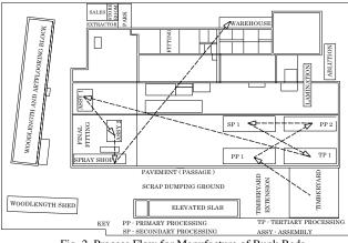
Fig. 2. Process Flow for Manufacture of Bunk Beds
