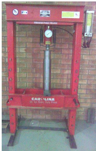
Fig. 2: 55 ton heavy duty Carolina hydraulic press with biomass compaction mold
