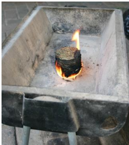
Fig. 6: Combustion behavior of typical loose biomass briquette
