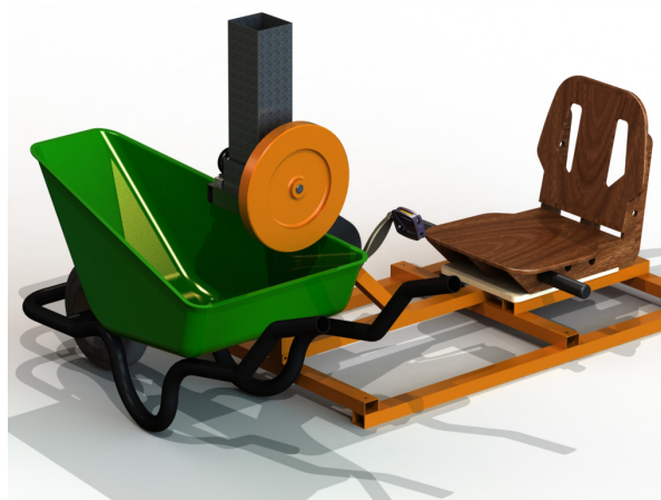
FIGURE 5 - Human-powered shredder prototype | rendering, 2015. (Courtesy of Peter H Harrison)
