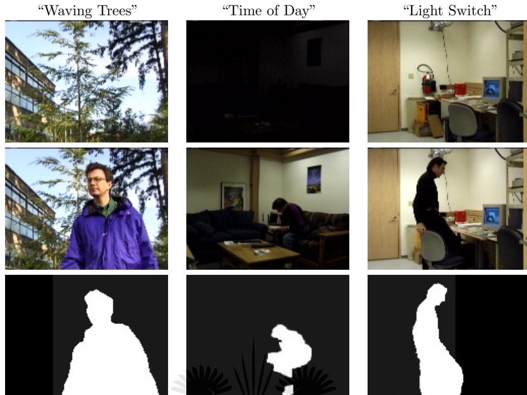
FIGURE 4.3: Three sequences from the Wallflower dataset. The top row represents the first training image while the middle row represents one of the images that will be evaluated. The bottom row shows one of the hand-segmented images that will be used as a ground truth in our experiments [73].
