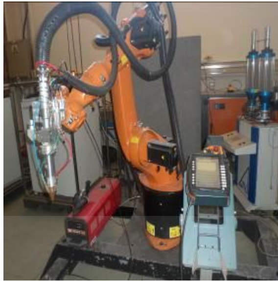
Figure 3. 1: Laser metal deposition machine connected to kuka robot with coaxial nozzle
