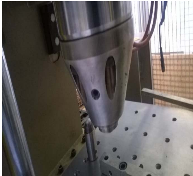
Figure 2: a pinless tool across the surface of the material for all the experiments.
