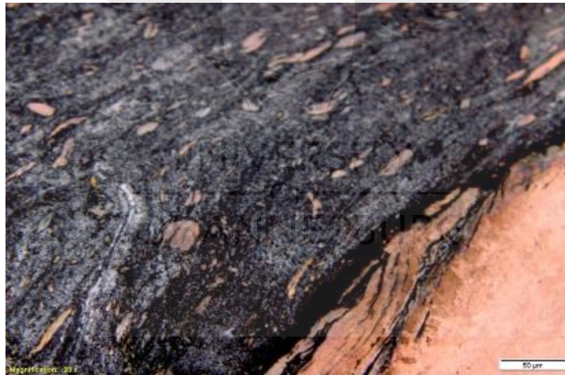
Welds produced at 800 rpm, 1 mm shoulder plunge depth using a flat pin and flat shoulder tool
