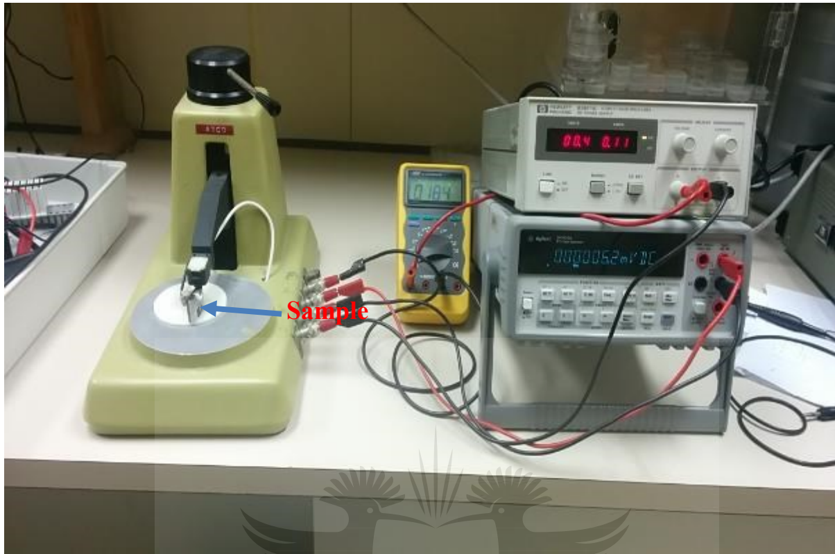
Figure 3-8 Experimental set-up for electrical resistance measurement
