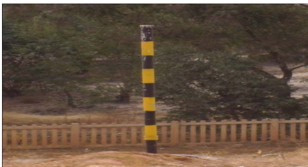
Fig. 8: Methane gas monitor at Luipaardsvlei landfill site
