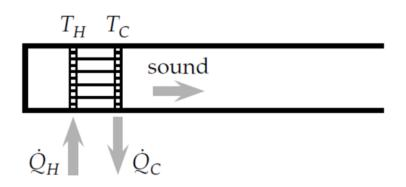
Figure 1: Thermoacoustic engine or prime mover
