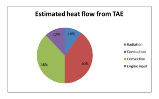
Figure 2: Heat flows from the power supply partitioned by the losses from radiation, conduction, convection and the power input
