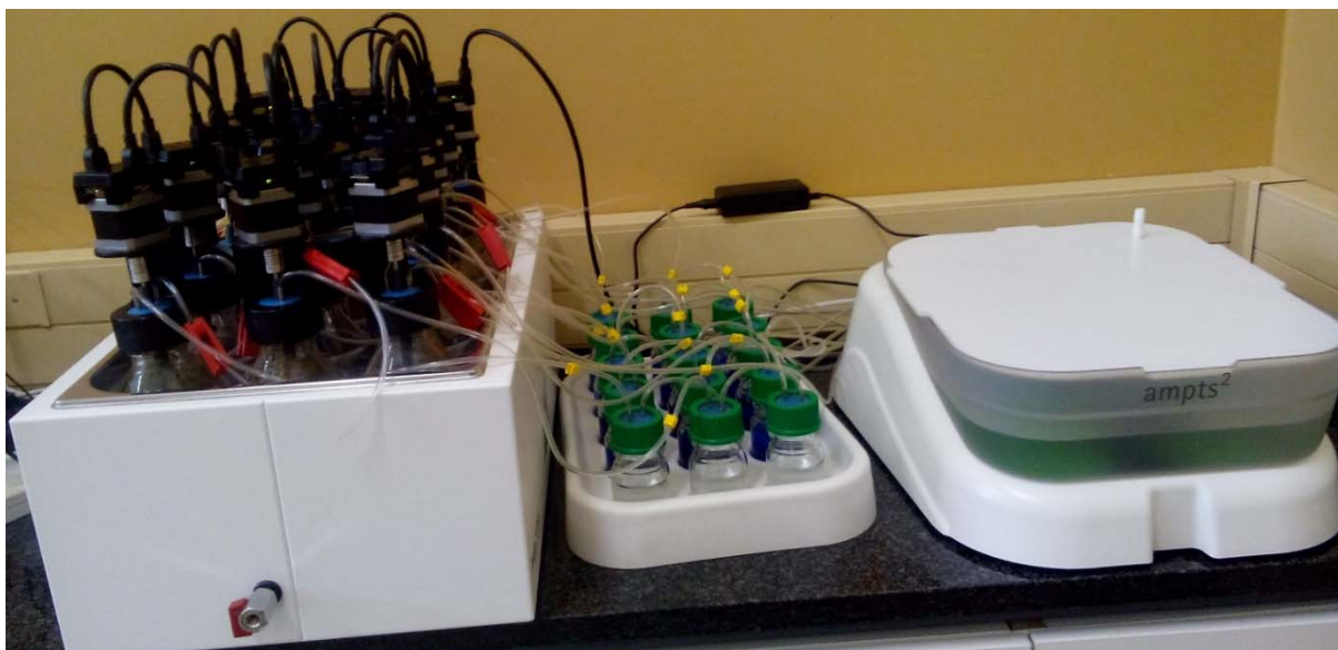
Fig. 1: Bioprocess AMPTS II experimental setup for BMP analysis
