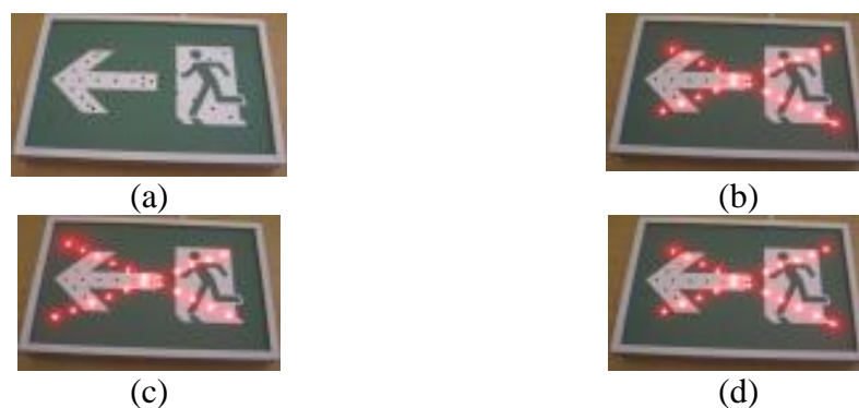
Figure 6: The ADSS implemented within the green running man signage concept demonstrating route negation.
