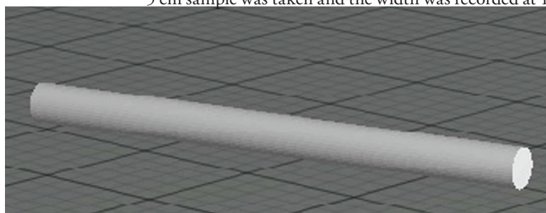
Figure 2. A rendered image of the implant of fixed dimensions 40 mm length and 3 mm diameter.
