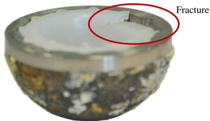
Figure 2-10: Fracture occurred at Polyethylene cup of a total hip prosthesis
