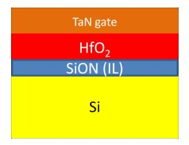
Fig. 4.5 Schematic of the HfO<sub>2</sub>/SiON gate stack
