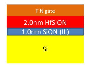
Fig. 4.14 Schematic illustration of the 2.0nm TiN/  $HfO_2$ / SiO<sub>2</sub> gate stack
