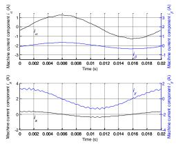
**Fig. 5.57:** Machine current components in the first ( $\alpha$ - $\beta$ ) and the second (*x*-*y*) plane.
