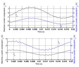
**Fig. 5.58:** Machine current components in the first  $(\alpha -\beta)$  and the second (x-y) plane.
