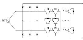
Fig. 2.4: Modified hybrid third harmonic injection rectifier.
