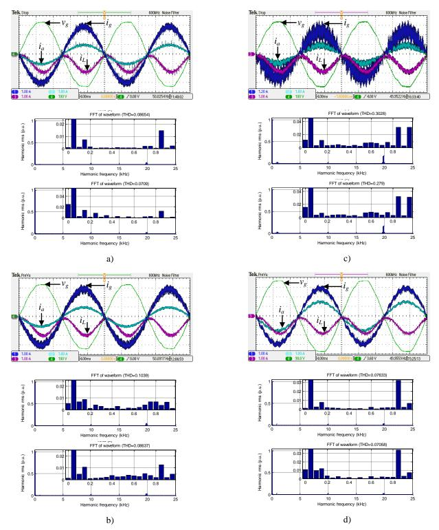
**Fig. 5.34:** Single-phase V2G with: a) asymmetrical nine-phase, b) asymmetrical six-phase, c) symmetrical six-phase and d) five-phase machine. The oscilloscope traces show grid voltage  $v_g$ , grid current  $i_g$ , machine phase *a* current  $i_a$  and battery charging current  $i_L$ . Current spectra are given for grid current  $i_g$  (upper graphs) and machine phase *a* current  $i_a$  (lower graphs).
