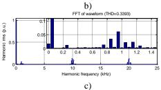
**Fig. 5.54:** a) Grid currents  $i_{ag}$ ,  $i_{bg}$  and  $i_{cg}$ , b) spectrum of grid current  $i_{bg}$ , c) spectrum of grid current  $i_{cg}$ .
