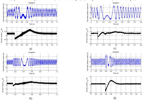
**Fig. 6.5:** Machine phase *a* current and battery discharging current during the reversal transient: a) nine-phase machine with  $i_{q \max}^* = 2.5$ A (-1000 to 1000 rpm), b) asymmetrical six-phase machine with  $i_{q \max}^* = 2.5$ A (-1000 to 1000 rpm), c) symmetrical six-phase machine with  $i_{q \max}^* = 3$ A (500 to -500 rpm), d) five-phase machine with  $i_{q \max}^* = 9$ A (800 to -800 rpm).
