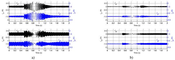
Fig. 6.7: Nine-phase machine current components in parasitic planes: a) harmonic elimination is disabled, b) harmonic elimination is enabled.
