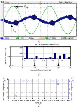
**Fig. 5.59:** a) Grid phase voltage  $v_{ag}$ , grid current  $i_{ag}$ , b) spectrum of grid current  $i_{ag}$ , c) grid current components  $i_{dg}$  and  $i_{qg}$ .
