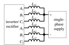
Fig. 3.5: Configuration for single-phase charging through a symmetrical or asymmetrical six-phase machine with two isolated neutral points.
