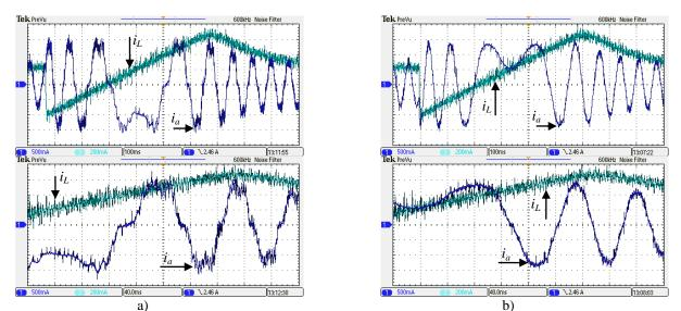
**Fig. 6.6:** Zoomed-in representation of the nine-phase machine's phase *a* current during the transient: a) harmonic elimination is disabled, b) harmonic elimination is enabled. Graphs also contain battery discharging current.
