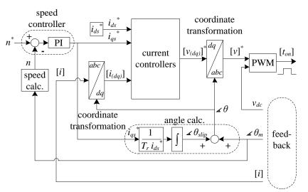
Fig. 6.1: RFOC control algorithm for multiphase machines
