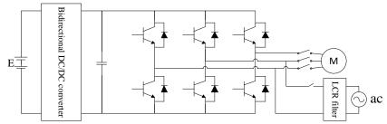
Fig. 2.17: Integrated battery charger using two legs of the inverter.
