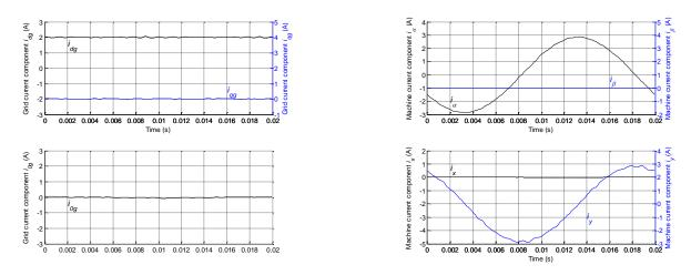
Fig. 5.26: Grid current components (on the transformer secondary side).
