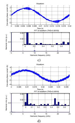
**Fig. 6.3:** Steady state operation of: a) nine-phase machine at 1000 rpm,  $i_d^* = 1.5$ A, b) asymmetrical six-phase machine at 1000 rpm,  $i_d^* = 3$ A, d) five-phase machine at 800 rpm,  $i_d^* = 4.5$ A. Index *s* in stator current component symbols is omitted.
