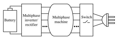
Fig. 1.1: Basic structure of an on-board integrated multiphase battery charging system.
