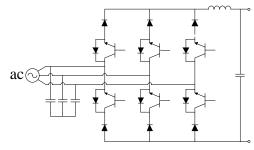
Fig. 2.8: Active six-switch buck PFC rectifier.
