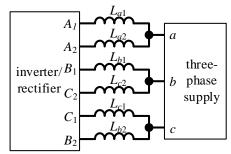
Fig. 3.10: Configuration for three-phase charging through a symmetrical or asymmetrical six-phase machine.
