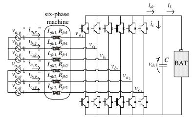
Fig. 5.3: Equivalent scheme of the six-phase topologies with supply as in Fig. 5.1.
