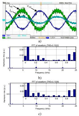
**Fig. 5.45:** V2G mode: (a) CH1 - grid phase voltage  $v_{ag}$  (150V/div), CH4 - grid phase current  $i_{ag}$  (1A/div) and CH2 - machine phase current  $i_a$  (1A/div) waveforms, (b) grid phase current and (c) machine phase current spectra - oscilloscope recordings and FFTs of measured variables.
