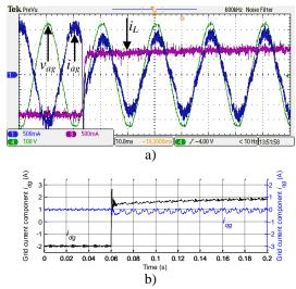
**Fig. 5.74:** a) Grid voltage  $v_{ag}$ , grid current  $i_{ag}$  and battery charging current  $i_L$ , b) grid current components  $i_{dg}$  and  $i_{qg}$ .
