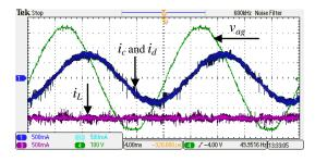
**Fig. 5.72:** Grid voltage  $v_{ag}$ , machine currents  $i_c$  and  $i_d$ , battery charging current  $i_L$ .
