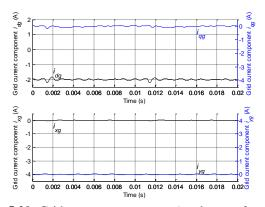
Fig. 5.20: Grid current components (on the transformer secondary side).
