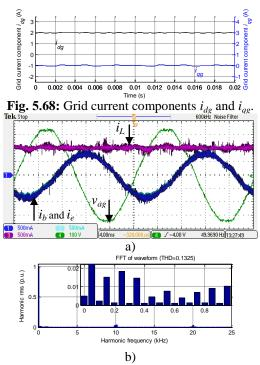
**Fig. 5.69:** a) Grid voltage  $v_{ag}$ , machine currents  $i_b$  and  $i_e$ , battery charging current  $i_L$ , b) spectrum of machine current  $i_b$ .
