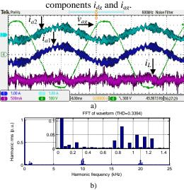
**Fig. 5.62:** a) Grid phase voltage  $v_{ag}$ , machine currents  $i_{a1}$ ,  $i_{a2}$  and battery charging current  $i_L$ , b) spectrum of grid current  $i_{a1}$ .
