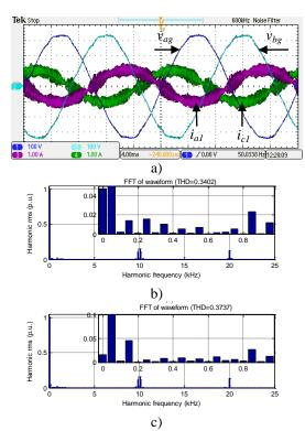
**Fig. 5.19:** a) Grid phase voltages  $v_{ag}$ ,  $v_{bg}$  and machine currents  $i_{a1}$ ,  $i_{c1}$ , b) spectrum of machine current  $i_{a1}$  c) grid current  $i_{ag}$  spectrum.
