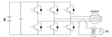
Fig. 2.20: Charger using all three phase windings of the motor.
