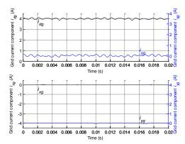
Fig. 5.16: Grid current components (on the transformer secondary side).
