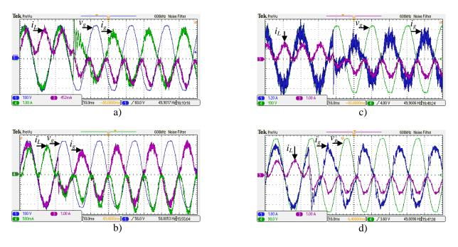
**Fig. 5.35:** Transient from charging into V2G mode of operation with: a) asymmetrical nine-phase, b) asymmetrical six-phase, c) symmetrical six-phase and d) five-phase machine. The oscilloscope traces show grid voltage  $v_g$ , grid current  $i_g$ , and battery charging current  $i_L$ .
