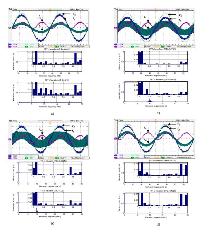
**Fig. 5.33:** Interleaved single-phase charging with: a) asymmetrical nine-phase, b) asymmetrical six-phase, c) symmetrical six-phase and d) five-phase machine. The oscilloscope traces show grid voltage  $v_g$ , grid current  $i_g$ , machine phase *a* current  $i_a$  and battery charging current  $i_L$ . Current spectra are given for the grid current  $i_g$  (upper graphs) and machine phase *a* current  $i_a$  (lower graphs).
