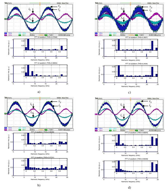
Fig. 5.32: Single-phase charging with: a) asymmetrical nine-phase, b) asymmetrical six-phase, c) symmetrical six-phase and d) five-phase machine. The oscilloscope traces show grid voltage  $v_g$ , grid current  $i_g$ , machine phase *a* current  $i_a$  and battery charging current  $i_L$ . Current spectra are given for the grid current  $i_g$  (upper graphs) and machine phase *a* current  $i_a$  (lower graphs).
