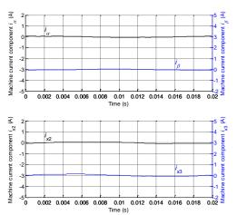
**Fig. 5.38:** Machine current components in inactive planes ( $i_{\alpha}$ ,  $i_{\beta}$ ,  $i_{x2}$ , and  $i_{x3}$ ), obtained within the controller after machine's measured phase currents are
