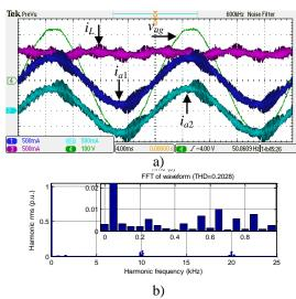
**Fig. 5.55:** a) Grid phase voltage  $v_{ag}$ , machine currents  $i_{a1}$ ,  $i_{a2}$  and battery charging current  $i_L$ , b) spectrum of grid current  $i_{a1}$ .
