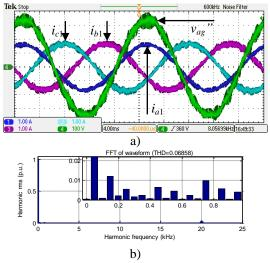
**Fig. 5.25:** a) Transformer secondary phase voltage  $v_{ag}$  and machine currents  $i_{a1}$ ,  $i_{c1}$  and  $i_{b1}$ , b) machine current  $i_{a1}$  spectrum.
