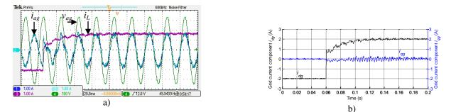
**Fig. 5.31:** Transient from V2G ( $i_d^* = -2A$ ) into the charging mode ( $i_d^* = 2A$ ): a) grid phase voltage  $v_{ag}$ , grid current  $i_{ag}$  (dark blue trace), machine current  $i_{a1}$  (light blue trace) and battery charging current  $i_L$ , b) grid current components  $i_{dg}$  and  $i_{qg}$ .
