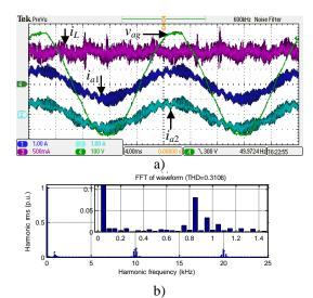
**Fig. 5.56:** a) Grid phase voltage  $v_{ag}$ , machine currents  $i_{a1}$ ,  $i_{a2}$  and battery charging current  $i_L$ , b) spectrum of grid current  $i_{a1}$ .
