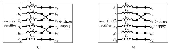
**Fig. 3.4:** Connection for the charging mode of operation of: a) an asymmetrical six-phase machine to the asymmetrical six-phase voltage source (no field production in the rotor), b) a symmetrical six-phase machine to the symmetrical six-phase source (a pulsating field exists in the rotor).
