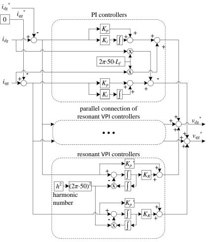
Fig. 5.13: Current control algorithm for the three-phase charging process.
