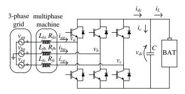
Fig. 5.11: Equivalent scheme of chargers supplied from three-phase mains.
