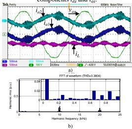
**Fig. 5.61:** a) Grid phase voltage  $v_{ag}$ , machine currents  $i_{a1}$ ,  $i_{a2}$  and battery charging current  $i_L$ , b) spectrum of grid current  $i_{a1}$ .
