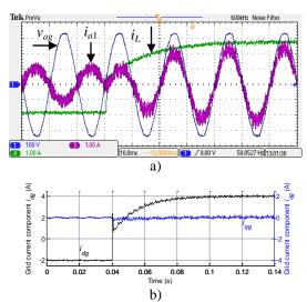
**Fig. 5.23:** Transient from V2G  $(i_d^* = -2A)$  into the charging mode  $(i_d^* = 4A)$ : a) grid voltage  $v_{ag}$ , machine phase current  $i_{a1}$  and battery charging current  $i_L$ , b) grid current components  $i_{dg}$  and  $i_{qg}$ .
