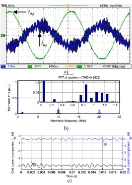
**Fig. 5.60:** a) Grid phase voltage  $v_{ag}$ , grid current  $i_{ag}$ , b) spectrum of grid current  $i_{ag}$ , c) grid current  $a_{ag}$ , c) grid current
