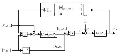
Fig. 4.6: Matrix representation of the model in decoupled domain.
