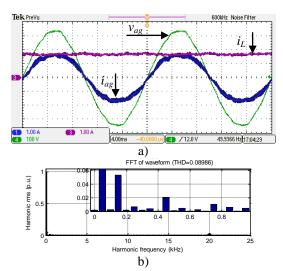
**Fig. 5.24:** a) Grid voltage  $v_{ag}$ , grid current  $i_{ag}$ , and battery charging current  $i_L$ , b) grid current spectrum.
