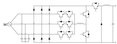
Fig. 2.10: Combination of the active filter third-harmonic injection rectifier and the dc-dc buck converter.
