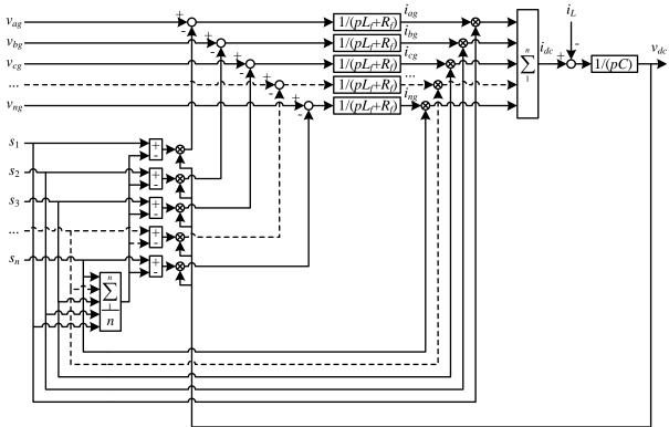
Fig. 4.3: Block diagram of the multiphase VSR in terms of phase variables (p stands for the differentiation operator).
