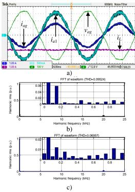
**Fig. 5.28:** a) Grid phase voltage  $v_{ag}$ , grid current  $i_{ag}$ , machine current  $i_{a1}$  and battery charging current  $i_L$ , b) grid current spectrum, c) machine current spectrum.
