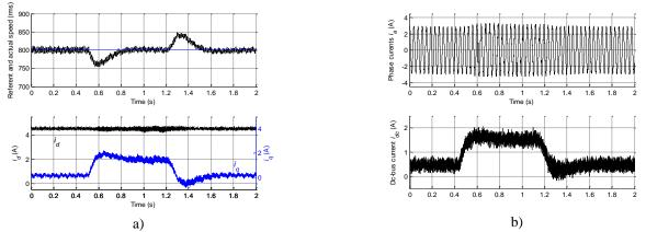
**Fig. 6.8:** Five-phase machine's load rejection transient: a) reference and measured speed, and stator current components in the first plane, b) machine phase *a* current and battery charging current.
