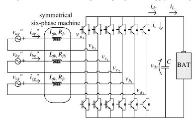
Fig. 5.4: Equivalent scheme of the symmetrical six-phase topology with supply as in Fig. 5.2 (covered in section 5.2.3).
