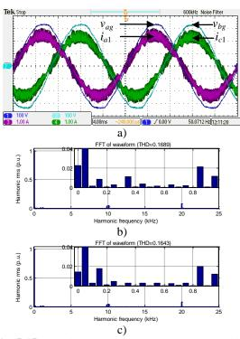
**Fig. 5.15:** a) Grid phase voltages  $v_{ag}$ ,  $v_{bg}$  and machine currents  $i_{a1}$ ,  $i_{c1}$ , b) spectrum of machine current  $i_{a1}$  c) grid current  $i_{ag}$  spectrum.
