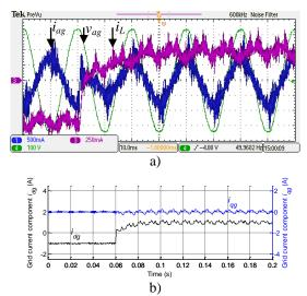
**Fig. 5.65:** a) Grid phase voltage  $v_{ag}$ , grid currents  $i_{ag}$ , and battery charging current  $i_L$ , b) grid current components  $i_{dg}$ , and  $i_{qg}$ .
