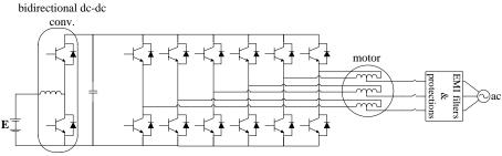
Fig. 2.27: Three-phase charger with access to the mid-point of each phase.
