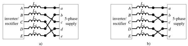
**Fig. 3.1:** a) Supply-to-machine connection according to the phase transposition rule (no field produced in the  $\alpha$ - $\beta$  plane, b) Configuration of connection with pulsating field in the  $\alpha$ - $\beta$  plane.
