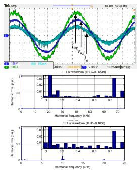
**Fig. 5.41:** Charging mode with interleaving: (a) CH1 - grid phase voltage  $v_{ag}$  (150V/div), CH4 - grid phase current  $i_{ag}$  (1A/div) and CH2 - machine phase current  $i_{a}$  (1A/div) waveforms, (b) grid phase current and (c) machine phase current spectra – oscilloscope recordings and FFTs of measured variables.
