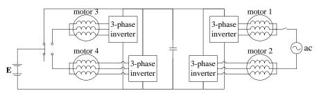
Fig. 2.21: Charger based on use of neutral point connection and four propulsion motors.
