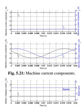
**Fig. 5.22:** Battery charging current  $i_L$  and machine speed.
