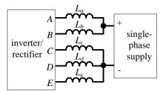
Fig. 3.7: Connection of a single-phase voltage supply to a five-phase machine.
