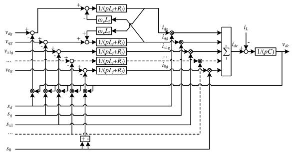
Fig. 4.7: Mathematical model of a multiphase VSR in the rotational reference frame.
