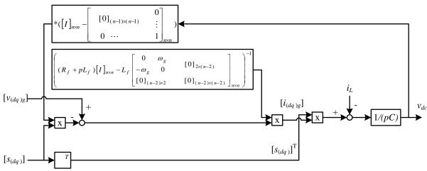
Fig. 4.8: Matrix representation of the model in the rotational reference frame.
