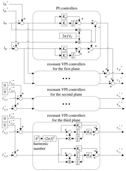
Fig. 6.2: Current controllers for propulsion mode of operation. Index *s* in stator current component symbols is omitted further on, for simplicity.
