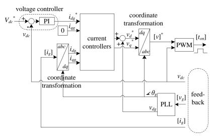
Fig. 5.12: VOC algorithm for the configuration from Fig. 5.11.
