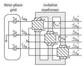
Fig. 5.2: An alternative symmetrical six-phase voltage supply (covered in section 5.2.3).
