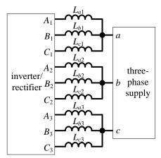
Fig. 3.8: Configuration for three-phase charging through a symmetrical or asymmetrical nine-phase machine with three isolated neutral points.
