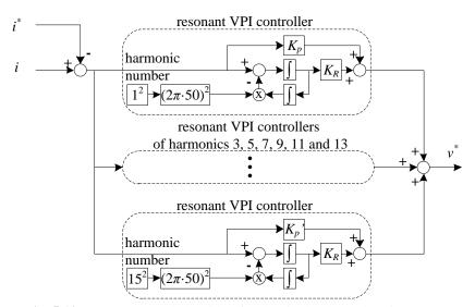
Fig. 5.10: Current control algorithm for the single-phase charging process.
