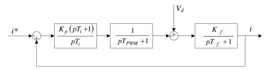
**Fig. 4.9:** Block diagram of the current control in an axis (*d* or *q*).
