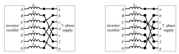
Fig. 3.3: Possible connections of a seven-phase machine to the seven-phase supply in charging mode.
