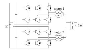
Fig. 2.19: Charger based on use of neutral points of the two motors.
