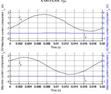
**Fig. 5.70:** Machine current components in the first ( $\alpha$ - $\beta$ ) and the second plane (*x*-*y*).
