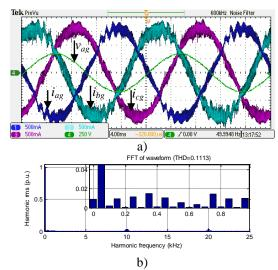
**Fig. 5.71:** a) Grid phase voltage  $v_{ag}$ , grid currents  $i_{ag}$ ,  $i_{bg}$ ,  $i_{cg}$ , b) spectrum of grid current  $i_{cg}$ .
