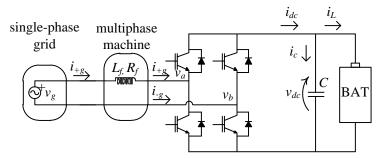
Fig. 5.8: Equivalent scheme of the charger supplied from single-phase mains.
