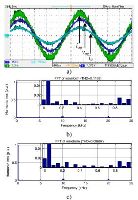
**Fig. 5.36:** Charging mode: (a) CH1 - grid phase voltage  $v_{ag}$  (150V/div), CH4 - grid phase current  $i_{ag}$  (1A/div) and CH2 - machine phase current  $i_a$  (1A/div) waveforms, (b) grid phase current and (c) machine phase current spectra – oscilloscope recordings and FFTs of measured variables.
