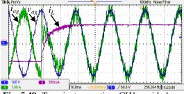
**Fig. 5.49:** Transient operation: CH1 - grid phase voltage  $v_{ag}$  (100V/div, blue trace), CH3 - dc-bus current  $i_{dc}$  (1A/div, purple trace), and CH4 - grid phase
