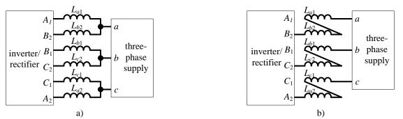
**Fig. 3.9:** Configuration for three-phase charging through: a) a symmetrical six-phase machine, b) a modified symmetrical six-phase machine.
