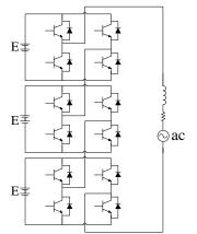
Fig. 2.18: One phase of a multilevel integrated charger.
