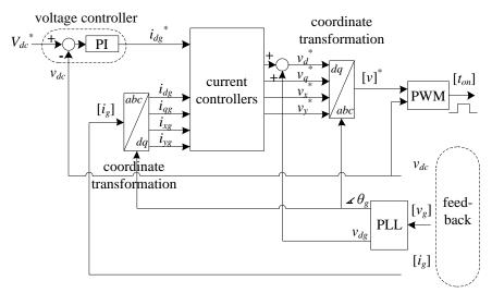
Fig. 5.5: VOC control algorithm for multiphase VSC.
