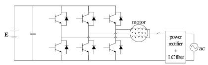
Fig. 2.22: Charger connected to the neutral point of a single motor.
