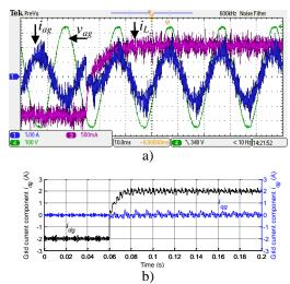
**Fig. 5.66:** a) Grid phase voltage  $v_{ag}$ , grid currents  $i_{ag}$ , and battery charging current  $i_L$ , b) grid current components  $i_{dg}$ , and  $i_{qg}$ .
