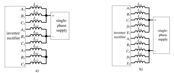
Fig. 3.6: Configuration for single-phase charging through: a) a symmetrical or asymmetrical nine-phase machine with three isolated neutral points, b) a symmetrical or asymmetrical ten-phase machine with two isolated neutral points.
