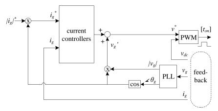
Fig. 5.9: Control algorithm for the single-phase charging/V2G process.
