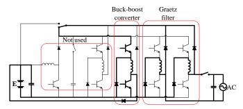
Fig. 2.23: Charger integrated with SRM drive.
