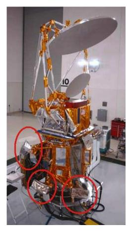
Figure 5.2: Schematic of SMEI in orbit. SMEI scans an area over a  $\sim 180^{\circ}$  range of the sky from three cameras looking outward from the Earth. Image from Jackson et al. (2004).
