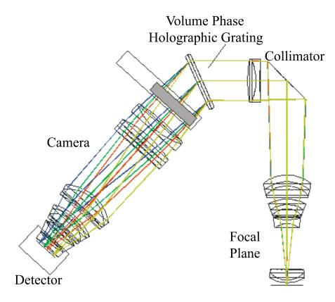
Figure 3.7: Schematic illustration of spectroscopy modes of RSS.
