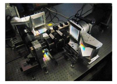
Figure 3.3: Part of FRODOSpec on an optical bench before shipping to site.
