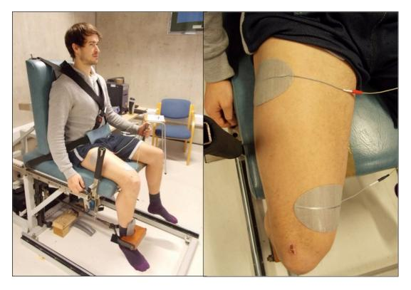
Figure 4.2. EMS experimental set up. Left: participant fully secured in the isometric chair. Right: placement of the electrodes used to deliver electrical stimuli.
