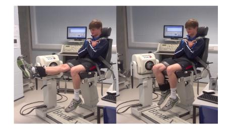
Figure 4.1. IKD experimental set up. Left: participant at full extension. Right: participant at full flexion.
