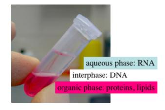
Figure 3.3. Example phase separation with TRI reagent.
