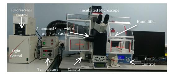
**Figure 3.13.** Annotated image of live imaging hardware used to perform live imaging experiments and fluorescence microscopy. Images are visualized via Leica Application Suite linked to the microscope.
