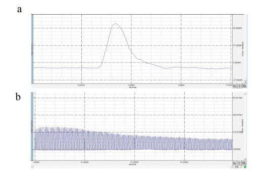
**Figure 4.3**. **a)** Example twitch feedback curve obtained from a 200 ms square wave pulse of 130 mA at a frequency of 1 Hz. **b)** Example fatigue data from two minutes repeated stimulation with 20 Hz, 200 msec square wave pulses every 750 msec. Representative output taken from AcqKnowledge software.
