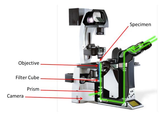
**Figure 3.11.** Schematic representation depicting the path of excitation and emission light in a fluorescence microscope. Excitation light (blue) is directed onto the sample via the objective. The fluorophore is then excited and emits fluorescence (green). The green light is passed through a prism filtering out light of other wavelengths and produces an image that can be seen through the eyepiece of camera of the microscope.
