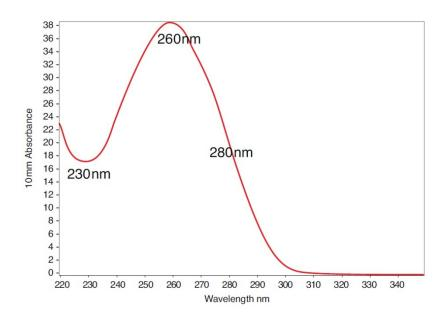
Figure 3.4. Example nucleic acid spectral image used to assess RNA sample quality.
