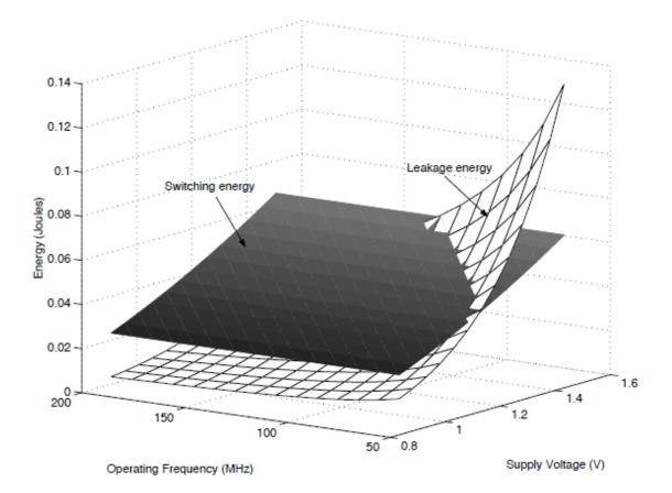
Figure 3.7 Comparison of leakage and switching energy in SA-1100 (Sinha and Chandrakasan 2000). The graph shows that the leakage energy begins to dominate as the processor's frequency is reduced. The leakage energy is linearly proportional to time irrespective of work being done or not. The simplest way to solve this is by powering off nodes which again requires time and energy overhead. A shutdown policy needs to consider the
