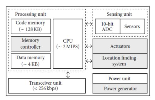
Figure 3. 8 Reference hardware platform architecture of a sensor node (Kuorilehto et al. 2005).
