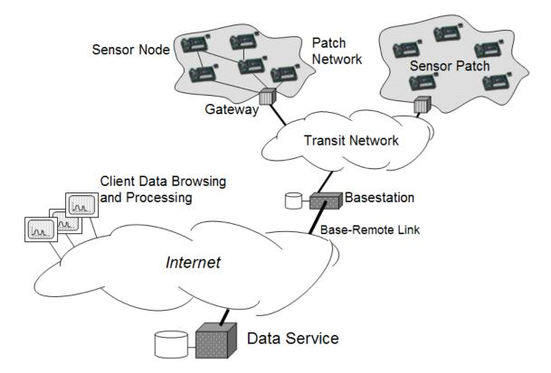
Figure 3. 11 System architecture for habitat monitoring (Mainwaring et al. 2002).
