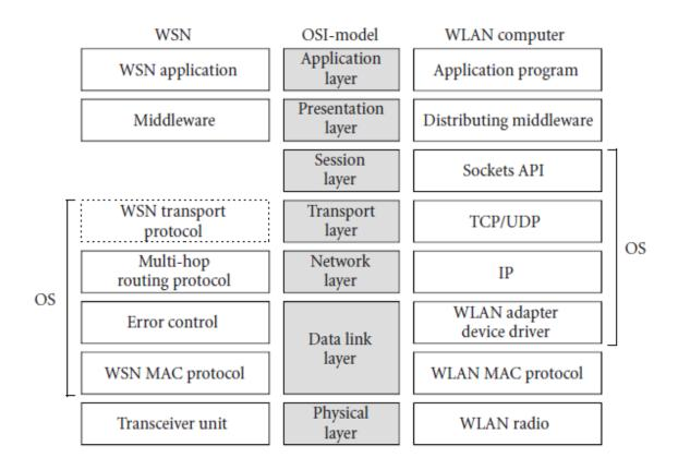
Figure 3. 10 OSI model, WSN, and distributed system in WLAN protocol layers (Kuorilehto et al. 2005).
