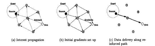
Figure 4.1 A simplified schematic for directed diffusion (Intanagonwiwat et al. 2000).
