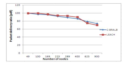
Figure 6. 16 Packet delivery ratio of C-BRALB vs. LEACH
