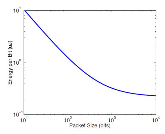
Figure 3. 6 The total radio energy per bit required to transmit packets of various sizes. The radio has a data rate of 1 Mbps, start-up time 466 µs, and the active transmitter electronics consume 220 mW (Min 2003).
