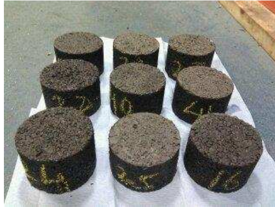
Figure 11: Subset of the bituminous mix samples prepared (control and rubberised)
