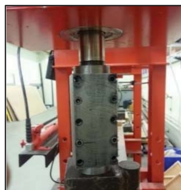
Fig. 4 Preparing of UCS test specimens
