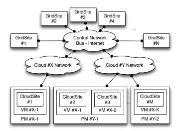
Fig. 7. Integrated GroudSim-DISSECT-CF networking
