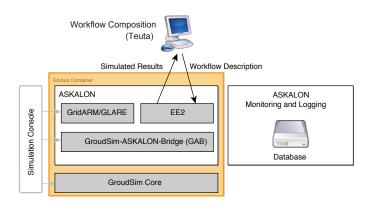
Fig. 1. The architecture of ASKALON
