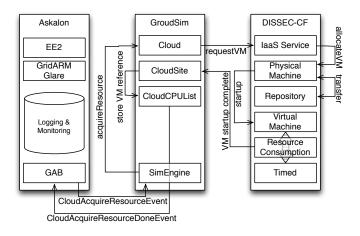
Fig. 5. Extended VM instantiation procedure
