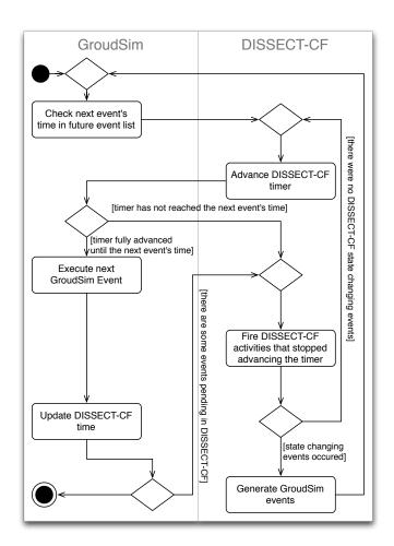
Fig. 4. Interaction between GroudSim and DISSECT-CF within the main event processing loop of GroudSim's simulation engine. *Remark: the diagram* only captures the processing of a single GroudSim event within the loop
