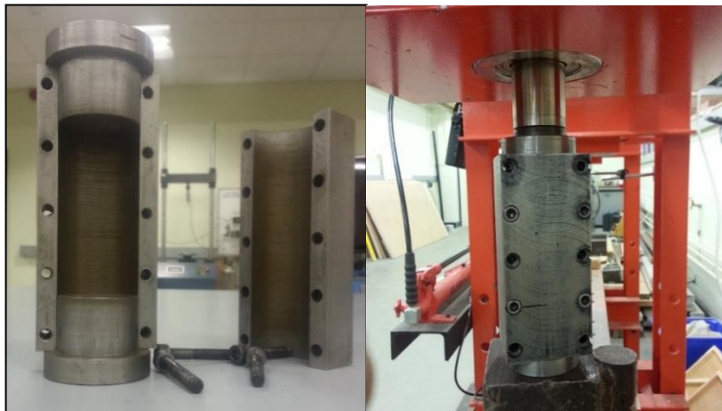
Figure 5. Constant volume mould and the hydraulic jack
