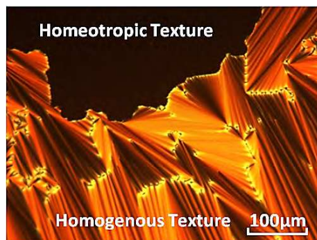
Fig. 4 The growth of the homogeneous texture in a 5 \mu\text{m} homeotropic aligned cell in the SmA_d phase at T - T_{ISmA_d} = -13^\circ\text{C} .
