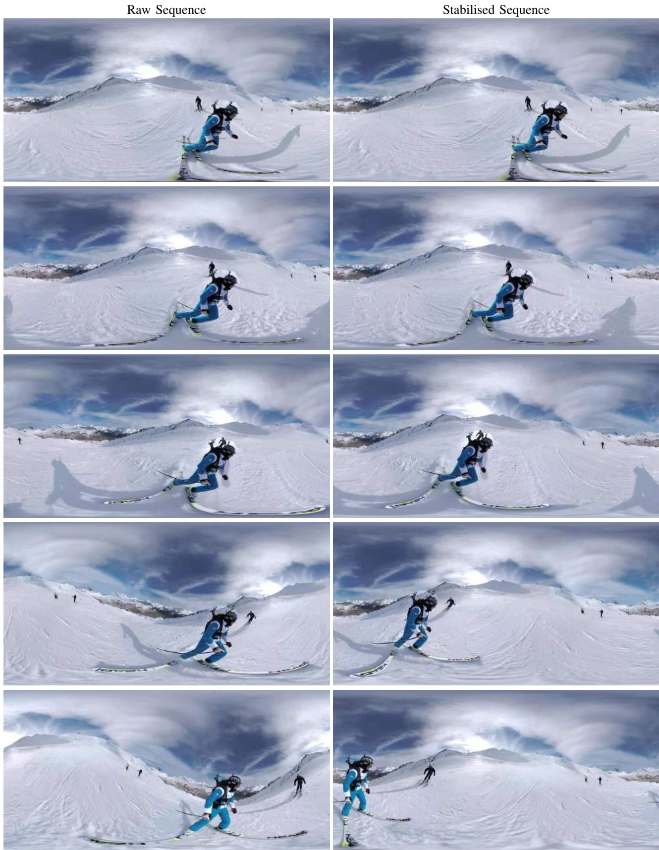
Fig. 5: Raw panoramic frames from spherical video sequence (left) and stabilised frames (right).
