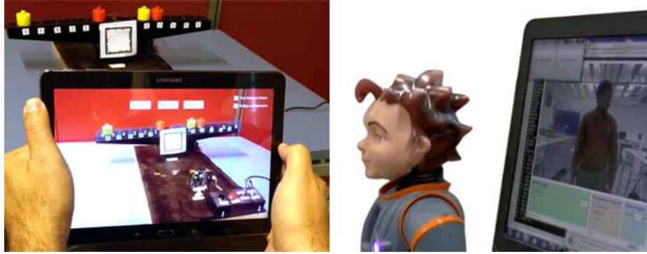
Fig. 4. The Zeno robot, the EASELscope and the Smart Balance Beam (SBB). Zeno acts as the embodiment of the STA and continuously interacts with the learner. Information about the task is displayed as augmented reality on top of the physical SBB.
