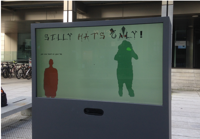
Figure 3. When a user performs the teapot gesture, their silhouette will get a silly hat. An animation in the bottom left of the screen demonstrates the gesture.
