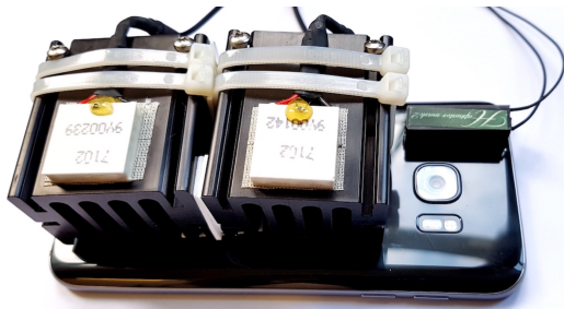
Figure 4: Phone with two 2cm 2 Peltier modules and a Haptuator Mk II on the back. Device rested in (stimulated) the palm.
