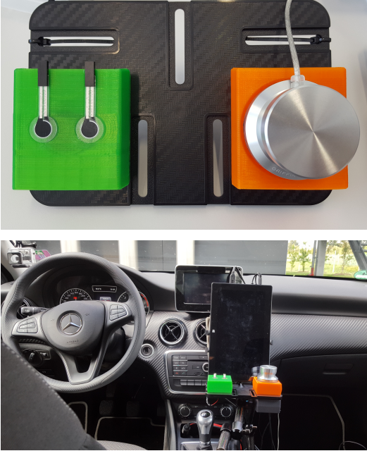
Figure 2. The force sensors and dial were placed on top of 3D printed cases (top). The touchscreen and hardware setup inside the car (bottom).
