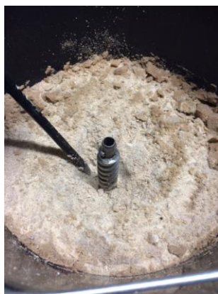
Figure 4: Drill Bit Seizure in Icy Regolith
